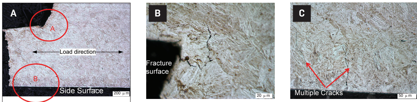
Fig. 10 — Cross section of the simulated CGHAZ charged from all four sides with loading: A — Low-magnification image; B — higher-magnification image of region A; C — higher-magnification image of region B.
