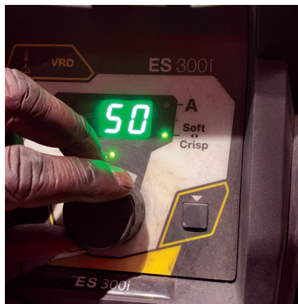
Fig. 3 — Professional-grade inverter power sources have controls for setting "crisp" or "soft" arc characteristics.
