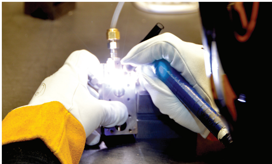
Fig. 2 — GTAW is possibly the most physically challenging manual welding process to perfect, as it requires the constant use of all four of the welder’s extremities.
