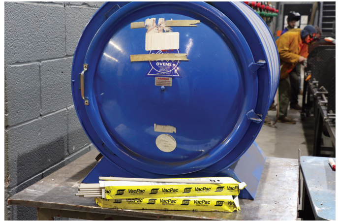
Fig. 2 — AWS D1.1 requires 7018 electrodes to be used fresh from hermetically sealed packages or stored in a rod oven.
