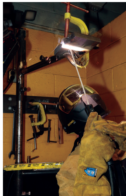
Fig. 4 — Position your head adjacent to the joint to see the electrode and its relationship to the weld pool.
