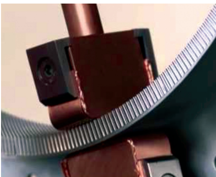
Fig. 3 — Honeycomb assembly is pressed between the two spot welding heads using controlled pressure and discharge power. (Photo courtesy of Aimtek/Soudax.)
