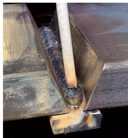
Fig. 6 — Alternate travel directions. Starting the new pass where the previous one ended fills in the "bowl" that tends to form at the end of the joint.
