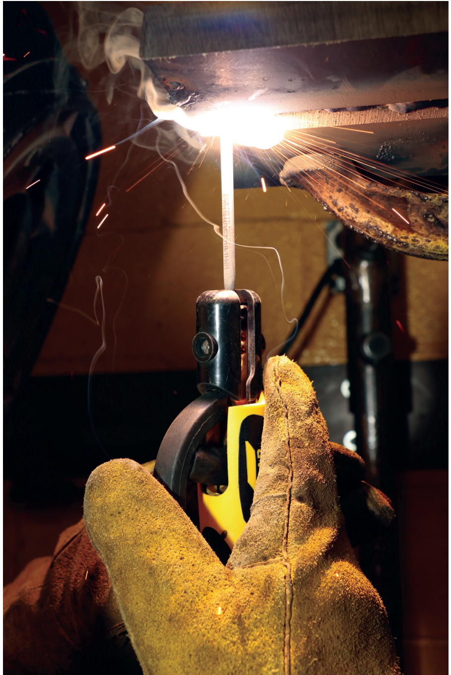
Holding the electrode perpendicular at the end of the plate minimizes arc blow.
