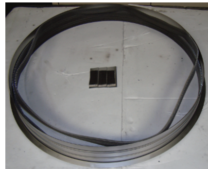
Fig. 6 — Improperly brazed honeycomb has pulled away from its substrate, as seen in this post-braze picture. (Photo courtesy of Aerovision.)
